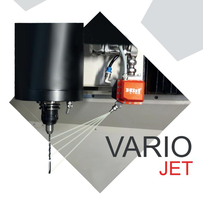
Automatic and targeted application of coolant!
